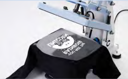
4 Tape the printed film on the t-shirt and press at 160°C /320 °F for 15 seconds.
