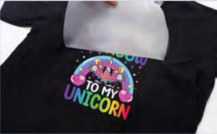
5 Cold Peel: Allow the film to cool, peel film away slowly; Hot Peel: Peel film away before it cools down.
